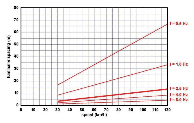
Figure 5.1: Critical luminaire spacing as function of driving speed for different flicker frequencies
