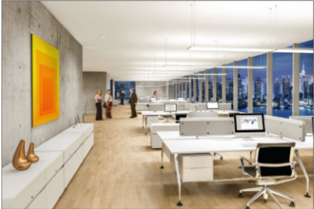
Figure 4: Visualisation of lighting solution 2 with Direct/Indirect luminaires with adjustable colour temperature and additional downlights
